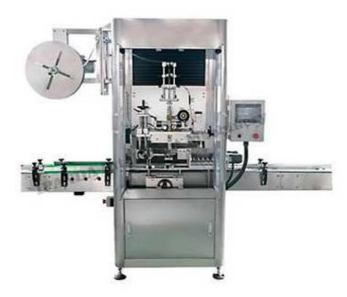
The machinery part adopts combination designing of modularization, and makes the machine reasonable. The height adjustment adopts motor fluctuating; it is convenient to replace the material. The special cutter head designing, make the film-rolling cut more exactly and reliably.
