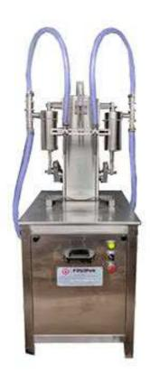
Semi automatic volumetric liquid filling machine is precision built on sturdy welded MS frame completely enclose in stainless steel sheet and doors are provided to facilitate the servicing of machine. Working on volumetric principle, the unit is made compact, versatile and enclosed in stainless steel elegantly matt finish body.
