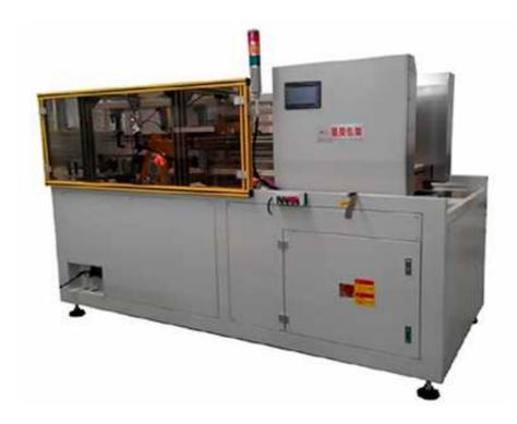
The KX-03 unpacking machine adopts a horizontal structure, which automatically completes the unpacking, forming, bottom bending, and the machine that completes the bottom tape sticking.
