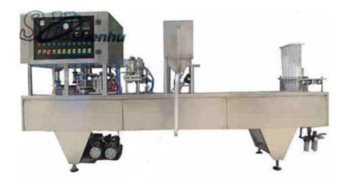
This series is made of stainless steel and is designed to meet the needs to can drinks into plastic bottles and cups of various shapes and the to seal, cut the edge, automatically control the temperature, print the production date and to sterilize with ultraviolet lay, it is mainly used in the industries like: drinks, brewing, medicine, seasoning, bean curd, jelly, pudding, fruit juice, milk, yoghourt and cold drinks
