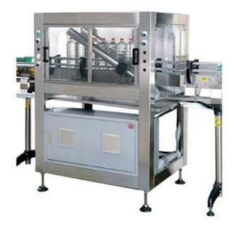
HAB Series bottle dryer is designed to remove excess water droplets from the surface of bottles. In a hot filling line, containers are spray cooled to a temperature close to ambient temperature for packaging purpose. HAB Series is integrated with low energy consumption but high volume output air blower for effective bottle drying. The length and number of air blowing tubes can be customized for different line specifications.
