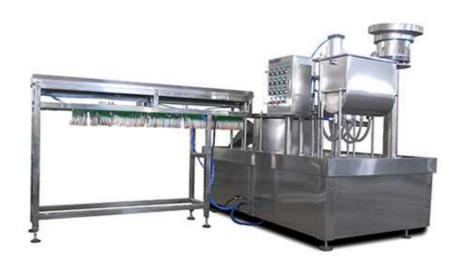
This machine is suitable for filling and capping spout pouch with liquid such as jelly, soy milk, milk, yogurt, pure water, fruit juice, ice cream, edible oil, seasoning, washing liquid, etc.
