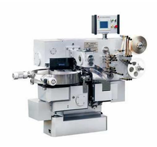
Wrapping machine for ball chocolate in foil wrap. The machine is suitable to wrap ball shaped choclate. The JH-G810 is adopted Indexing drives and cam transfer structure, be able to equip with a sorting station to eliminate sugar dust, chips and broken pieces. An efficient feeding is achieved by the approved plate feeding system. The length of packing material is controlled by the servo motor.
