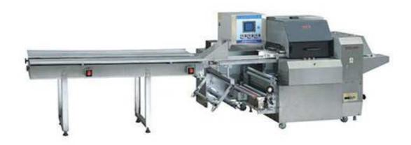
A quick change of product dimensions is possible by exchange of the wrapping units.
