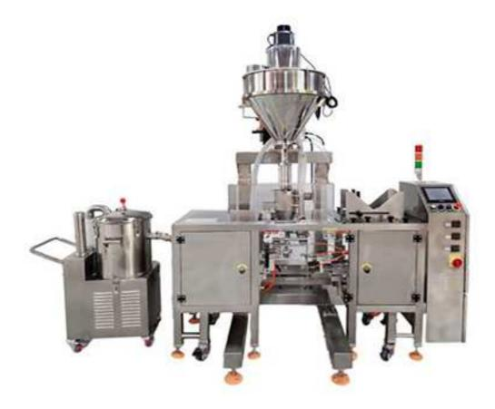
With different feeders changed to pack solid, liquid, thick liquid, powder and so on, Doypack machine is suitable for all kinds of the premade bags, such as pillow bag, 3-side, 4-side and 8-side quad seal bags (box pouch), kraft bags and spout bags ect, Product or packing pouch contact parts adopt stainless steel or other materials which accord with the food hygienic requirements, guarantee hygiene and security of the food
