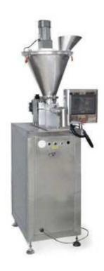
The machine is a semi-automatic series filling machine, horizontal screw device lifting table, round bucket and stirring device, PCC man-machine interface, servo motor drive, weighing module, Clamping bag weighing mode. 304 stainless steel, adapt to artificial bagging, bottles, boxes filling. Particularly suitable for a variety of mixed powder material filling, and special materials weighing packaging.
