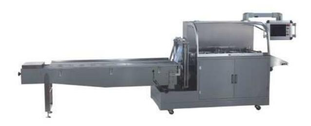
This machine is designed on basis of multi-function pillow packing machine and is suitable for packing warm cooling gel and similar product packaging design and development of products of domestic initiation.
