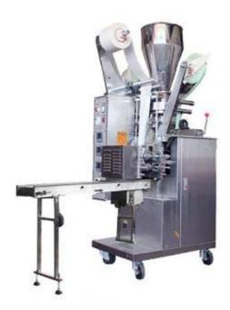
It is suitable for automatically packing dust tea products (filter bag), such as fragmental tea, medicinal tea, herb tea and so on. It is safe for the products and controlled by PLC. And different type has the different function.
