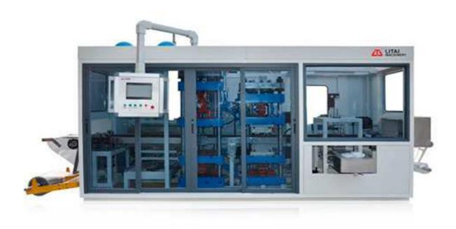
PET egg tray forming machine is using PP/PS/PVC/PET/HIPS material to make disposable plastic egg trays, lids, soap trays, plastic containers, pads, bowls and etc. It is full automatic driven by servo motor.
