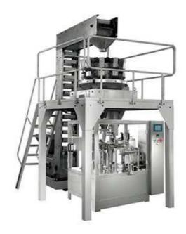
This line mainly installs rotary packing machine, combination weigher and Z-Conveyor, suitable for packing all kinds of grains and solids, such as candy, nuts, raisins, peanuts, melon seeds, potato chips, chocolate, biscuits and so on.
