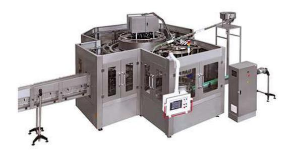
This machine is mainly used in edible oil and condiments production line, using flowmeter and weighing type filling usually. It has the advantages of high precision, no drip and leakage, and high automation. This machine is suitable for all kinds of bottled edible oil, condiments product, etc with production capacity ranges from 2000BPH to 20000BPH based on 500ml volume.
