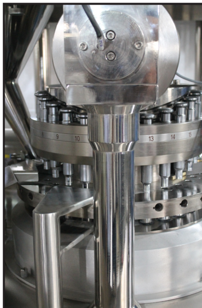
Main Compression with upper punch penetration
