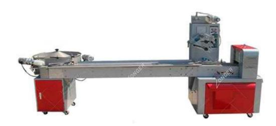
Our candy bar packaging machine is mainly used to pack candy, chocolate, cookies and other ordinary shapes. The machine has two feeding methods: automatic feeding and manual feeding.
