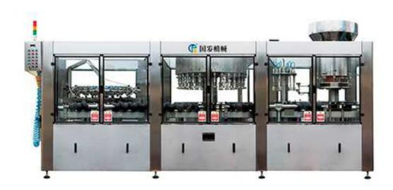
The principle of low-vacuum filling is adopted, and the bottle is filled against the wall to ensure that the liquid level is consistent after filling.
