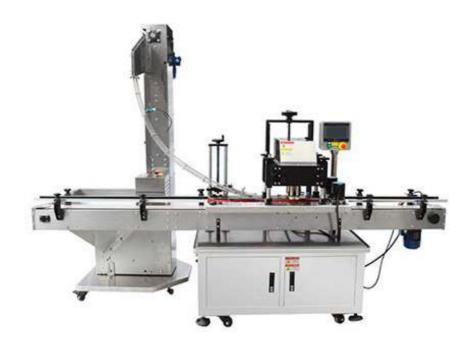
The capping machine can tighten the cap quickly and accurately to prevent the material from spilling out.
