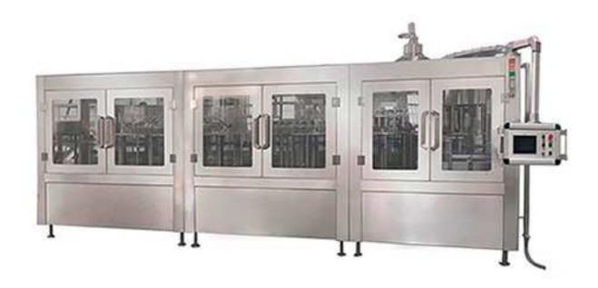
5-in-1 ultra clean filling system integrates two rounds of disinfectant rinsing, aseptic water rinsing, filling and capping. Filling temperature is 65-72°C no need to use the heat resistant bottle, therefore the bottle cost is reduced. As the filling temperature is lower, the saint are requirement and the microorganism control are stricter. Capacity: 6000-40000BPH.
