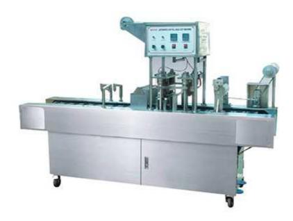
Automatic cup box filling and capping machine is suitable for the packaging of soy milk, milk yogurt, fruit juice drinks, mineral water and other beverage categories. Automatically complete cup dropping, filling, ultraviolet sterilization, photoelectric tracking, date printing, sealing, cutting, etc. The machine is made of stainless steel, with simple structure and reliable performance. It can be customized according to special requirements.
