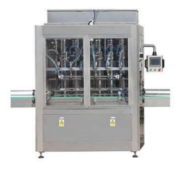
This sunflower oil filling machine, sunflower oil filler is design and manufacturing specially for filling engine oil, lube oil, gear oil and any other types of car oil, the oil filler is an extremely flexible filler, it is capable of filling any other liquids without corrosive.
