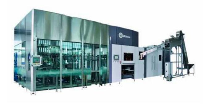
Blowing, filling and capping machine XLBFCGS6-035 is applied in the food, chemical and pharmaceutical industries to fill plastic bottles and cans.
