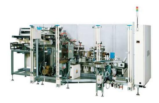
The CF210 cartoner neatly fills pouches into one-touch cartons automatically. This is a suitable solution for filling several retort pouches into cartons. Pouches which are accumulated at given number will be carefully placed in the cartons, without damaging the package and then flaps are tucked in. Either flat pouches or self-standing pouches can be handled.
