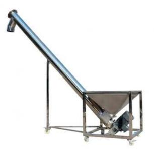
Screw conveyor is consisted of a screw, conveying pipe, drive motor, square feeding hopper, support frame and control panel. This machine material is stainless steel, which is anticorrosive and food grade. It can help convey powder or tiny granule materials from one place to reset position.
