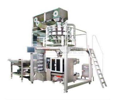
The multi-head weighing system has high accuracy and with the two servo driven packing machine, the whole machine system has high efficiency and high stability. Also the multi-head packing machine is in wide applications for varieties of products:
