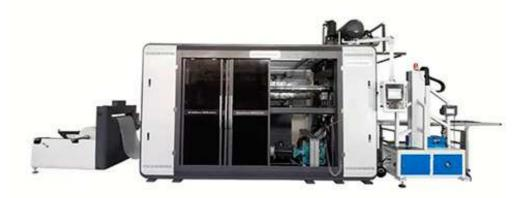
The cup making machine is Mainly for the production of variety plastic containers (jelly cups, drink cups, package containers, etc) with thermoplastic sheets, such as PP, PET, PE, PS, HIPS, PLA, etc.
