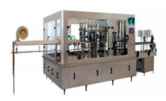
Juice Filling Machine/Juice Filling Production line Description: This RXGF series equipment is used in hot filling and sealing of green tea, black tea, wulong tea and fruit juice drink. The machine integrates washing, filling and capping together, the design is scientific and reasonable. Its appearance is beautiful. Its operation and operation is convenient.
