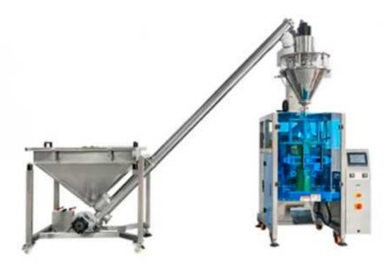
Dession powder packing machine is widely used in food factory, chemical factory, suitable for packing all kinds of powder product, such as, rice flour, coffee powder, sulfur powder, milk powder, seasoning powder.
