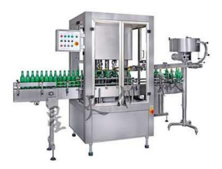
The YG-8 automatic capping machine (pressure plugging machine) is specially designed for the pressure lock sealing of the cylindrical bottles with plastic inner cover and the outer cover. It has strong adaptability to recycled bottles, stable and reliable performance and simple operation. The machine has reasonable design, high degree of automation, automatic cover and cover, and automatic removal and anti-cover device.
