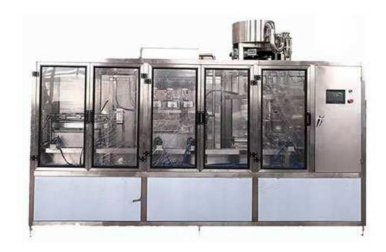
Linear Type Filling Machine Is Usually For Small Capacity Production Line. The Speed Is Up To 1000Bph. Bottles From 3L to 10L Are Optional. It Has a Compact Structure And Is Easy To Operate And Maintain. The Price Is Lower Than Rotary 3 in 1 Filling Machine.
