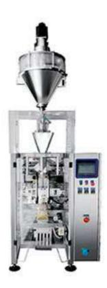
Economic VFFS machines provide simplicity and efficiency for food and non-food applications while using a roll of film to make bags. They specifically designed for the wrapping of a wide range of product types in medium to small-sized bags and capable of packing up to 100 bags per min maximum.
