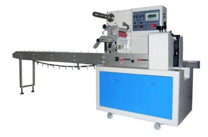
The MK-600D horizontal flow pack-wrapping machine accommodates a maximum film width of 600mm, making it ideal for wrapping items with regular shapes. Controlled using a dual inverter, the bag length setting is freely adjustable without having to interrupt the packaging process, thus saving packaging materials and money.
