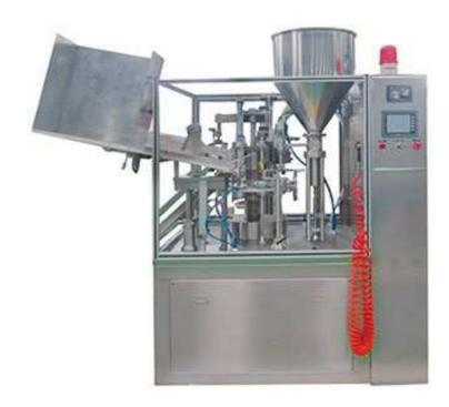
GZJ50 Tube Filling Machine is widely used in toothpaste, cosmetics, pharmaceutical cream category, food, shoe polish and viscose and other industries. It is applicable to aluminum-plastic, plastic hose packaging products filling, sealing and printing lot number. It can fill liquid material and cream material through special design and special filling device. It can be used independently, but also with automatic packaging machines and other equipment production lines.
