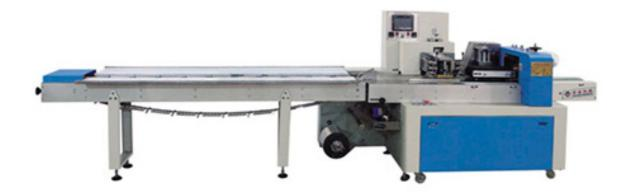
Suitable for packing all kinds of irregular solid, bulk, long strips and soft objects, just like, instant noodles, sausages and sockets switch clean ball, etc.
