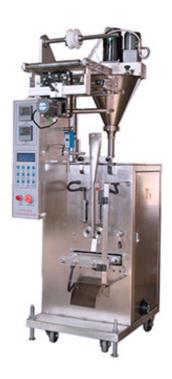
The process of measuring, bag-making, filling, sealing, printing and cutting can be done automatically.
