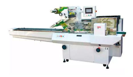
Thanks to the box motion end sealing system, the model is capable of covering a wide range of applications with less air packages and hermetic sealing. Flow pack machine for mooncakes, biscuits, cards, etc.
