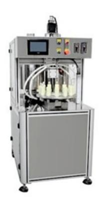
This machine is a kind of semi-auto filling machine for mascara and lip-gloss. The process section is including auto filling, automatic wipers inserting, brush inserting and capping device.
