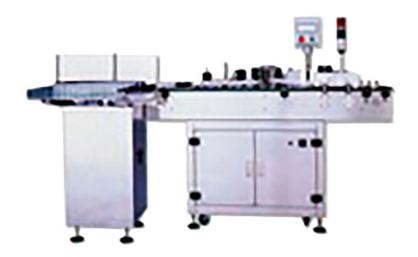
This machine is widely used for labeling of round containers in food, medicine, fine chemical and etc, such as oral liquid bottles, ampoule bottles, syringes, needle tube sleeves, batteries, hoses, cultural supplies and so on. This machine adopts servo motor for control. The human-machine touch screen is convenient and easy to operate; the rich failure display function can realize high-speed labeling.
