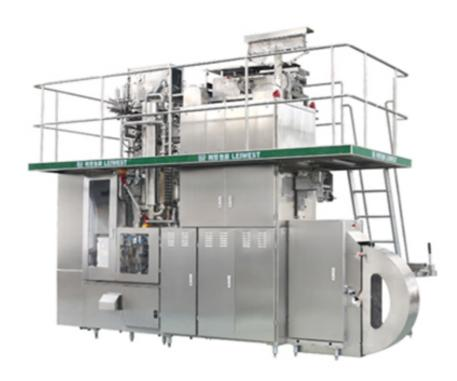
LWG-1 aseptic filling machine is used to fill pre-sterilized liquid product into packaging material in aseptic condition. The package was sealed and formed simultaneously to prolong the shelf life of the drinks.
