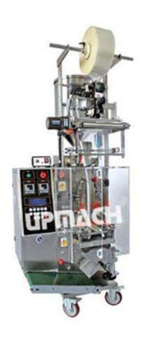
Liquid sachet filling machine is a vertical form fill seal (VFFS) machine that can be used for packaging of liquid, shampoo, lotion, oil, ketchup, soy source, jam, honey, disinfection water, alcohol gel, hand sanitizer gel, jelly and so on.
