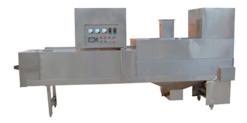
This machine is applied to dry, sterilize various glass bottles, such as oral liquor, clinical bottle and dropping bottle, and transfer by web sling (or chain). The speed of the web sling is adjustable.
