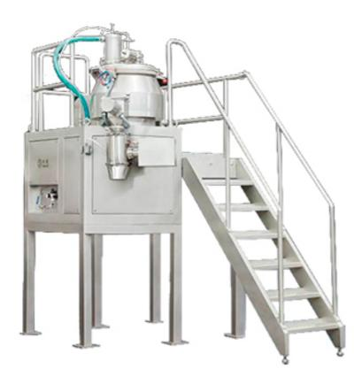
The GL series high shear mixer granulator is used in pharmaceutical solid dosage areas for mixing and granulation application as the primary processing equipment for a solid dosage production line. It is PLC controlled, and meets current GMP and pharmaceutical code regulations.
