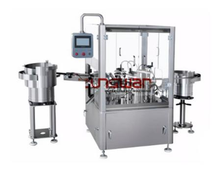
Mascara Filling &Plugging and Capping Machine with functions of automatic filling, loading brush and capping. The whole machine adopts PLC control, with the function of no bottle no filling, no brush no cover, easy operation and adjustment conveniently.
