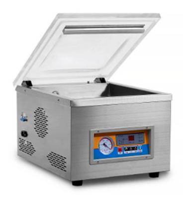
DZ300/PD Table type vacuum packing machine is featured by processing of vacuuming, sealing, cooling, which is used in vacuum packaging for the food, pharmaceutical, aquatic, chemical and electronic industries. It can prevent the products from oxidization and mildew, as well as corrosion and moisture, keeping the quality and freshness of the product over a prolonged storage time.
