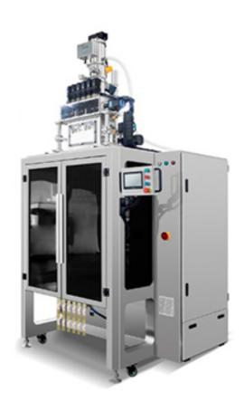
The multi lane packaging machine can simultaneously produce multi lane bags. The filling measurement system adopts a long screw filling device, which has the advantages of no blockage, higher accuracy (accuracy+-0.1 g when filling 1-5 grams), less dust, and avoids the powder stick packaging machine from clamping and sealing during the production process, resulting in loose sealing, air leakage, etc.
