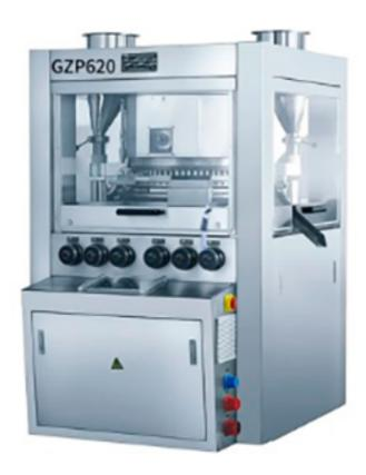
This machine is one kind of double side rotary tablet press machine, which can press granular materials into round shape tablet, irregular tablet or double-side engraved tablet.
