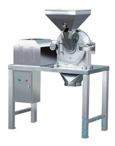
FG-300 High-efficiency Hammer Mill is extensively used in pharmaceutical, chemical, food and pesticide industries for pulverizing dry brittle materials.
