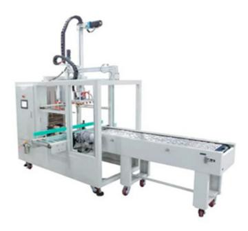
In the automatic packaging line, the packing machine is the core of the whole system. The packing machine is used to complete the transportation packaging, which is a kind of machinery that loads the packaged products into the carton according to a certain arrangement. P.L.C + touch screen control with missing bottle alarm stop, no bottle no packing safety device.
