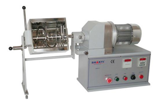
This Attachment fitted on special design stand. The power [Ribbon] mixer having horizontal half round bowl open on upper side with Vacuum tight top lid and specially designed mixing blade having two stages both right and left hand ribbon type mixing blades. The Bowl can be delivered with a double jacket for cooling or heating with water or Electric Heating system.
